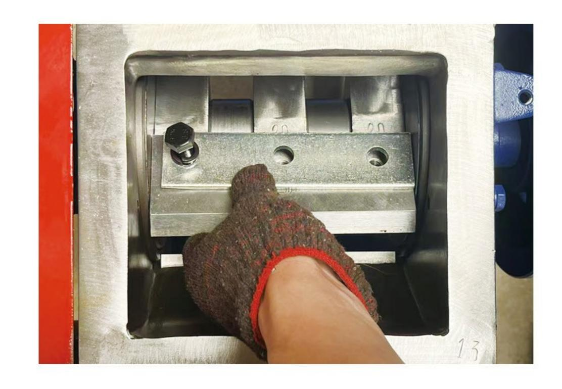
**For glass crusher:** Start with the left and right movable cutters on the same plane. Rotate the cutter holder to observe the distance between the movable edges and the front fixed cutter.
